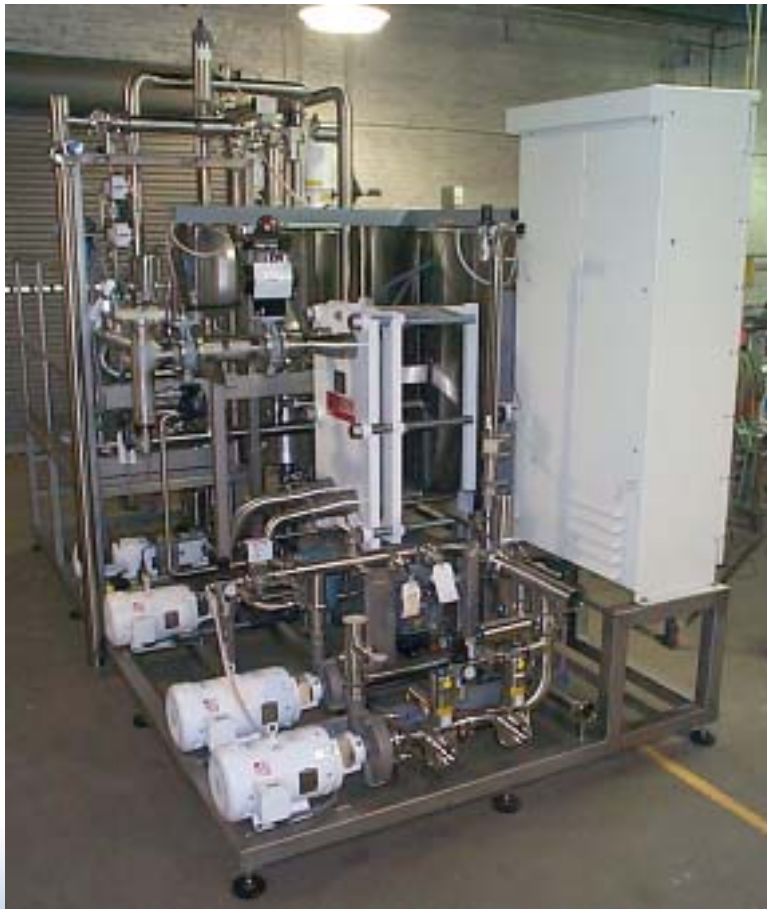
The DSI Water Blending System featuring an ozone injection system.
