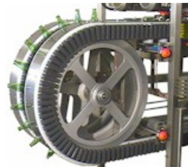
How containers are indexed for rinsing. Show with covers removed.
