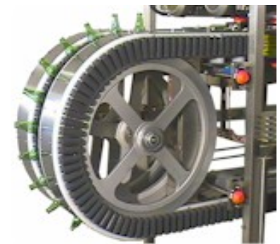
How containers are indexed for rinsing. Show with covers removed.
